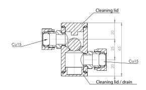
The Airfi Water Trap is designed for draining condensate from all small air handling units. The condensate water flows from the trap to the floor drain using a float within the product. The ball-shaped float prevents airflow back into the trap, making it silent.
